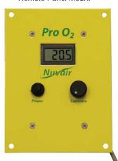
Please note: Never expose gas sensors to pressure or you may cause damage and/or false readings. Damaged sensors will not provide accurate gas analysis. Inaccurate gas analysis can lead to serious personal injury or death. Most gas analyzers can be used to analyze a regulated gas sample flow, the contents of a gas cylinder, or the flow from a regulator. The flow rate of gas must equal 0.5-5 L/min. To produce this flow, a flow restrictor and regulator may be required.
